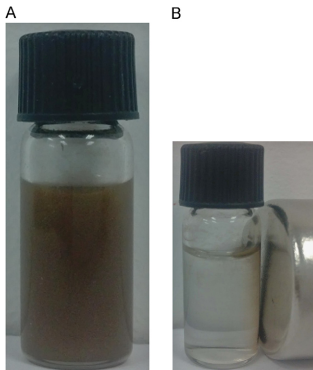
Fig. 3. Photos of: (A) aqueous dispersion of the magnetic \text{C8-Fe}_3\text{O}_4@\text{mSiO}_2 microspheres (B) after separation with a magnet for a few seconds.
